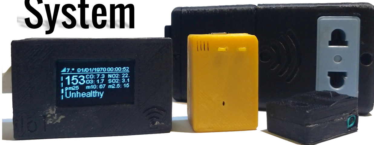
Light Box Image 1: Front view of the four IoT devices. (from left to right; display, temperature logger, button, and outlet)
