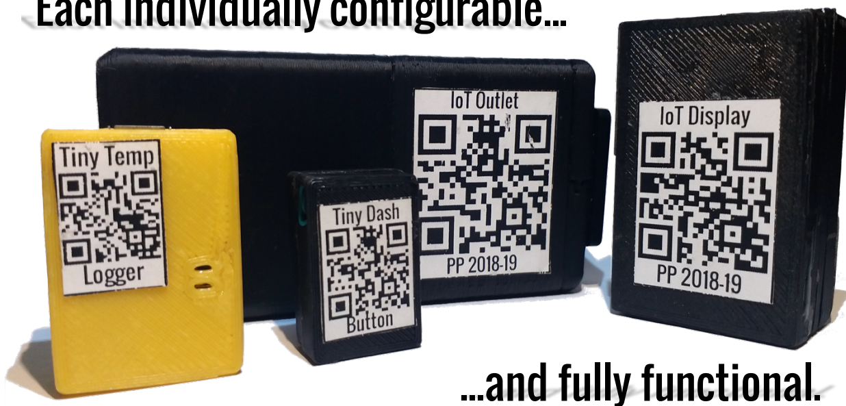
Light Box Image 2: Back view of the four IoT devices, showing the QR codes used for configuration.
