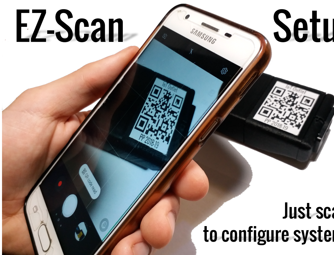
Light Box Image 4: Scanning of a QR code to quickly control and configure links/connections in IoT system.
