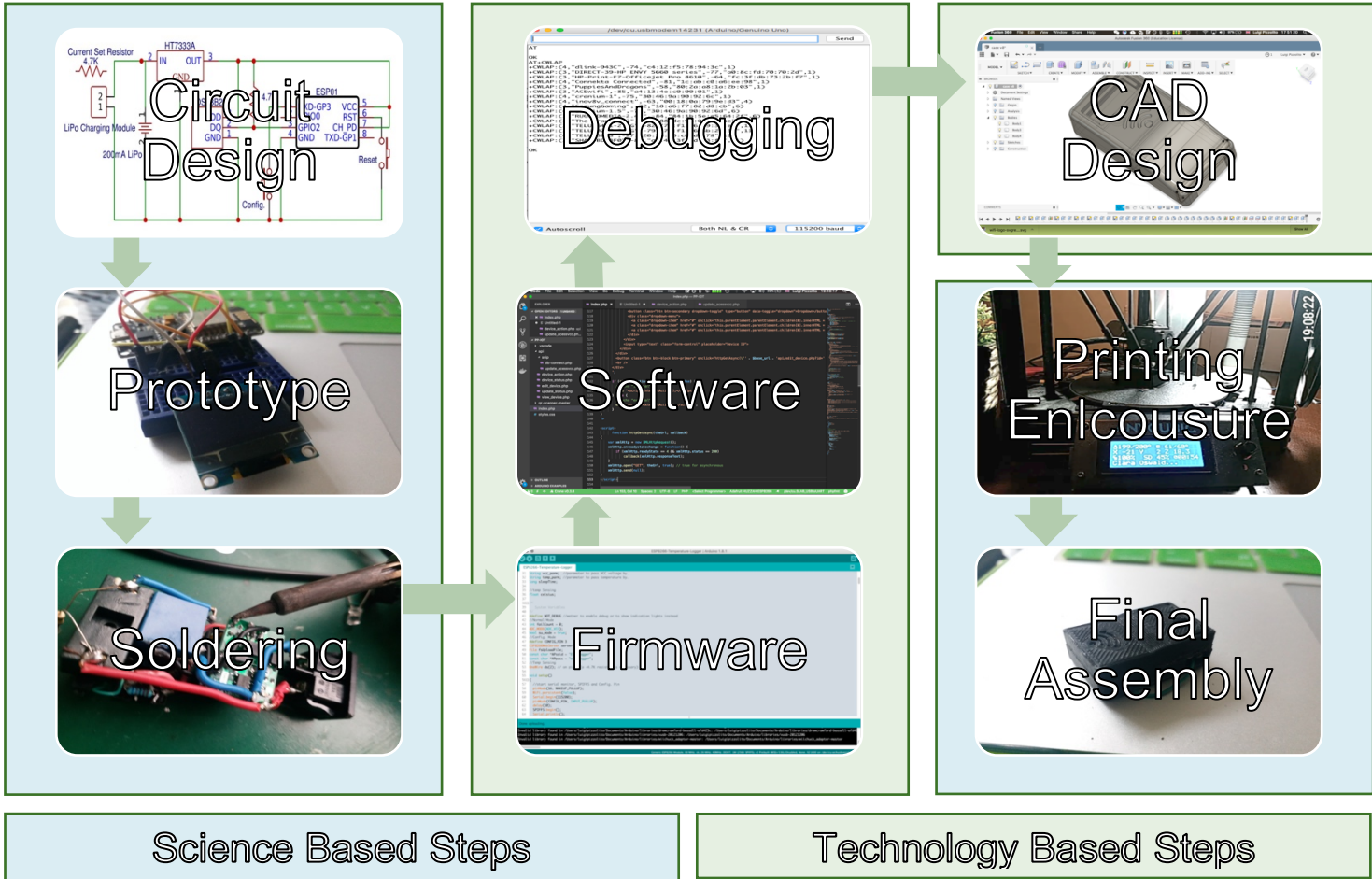
Diagram 9: Process of creating each IoT device... (4 of them)
